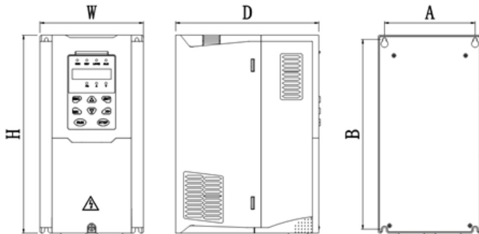
Fig. 5 – SIZE A to SIZE C Dimensions
