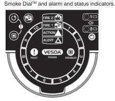
When the field service access door is open, the user has access to the RESET O DISABLE , Fire Test , AutoLearn and Instant Fault Finder functions. When the Instant Fault Finder function is activated, the Smoke Dial™ converts to a fault indicator, with the dial segment numbers corresponding to the faults listed below.
