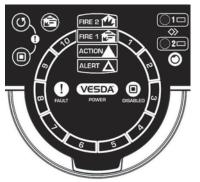
When the field service access door is open, the user has access to the RESET () DISABLE
