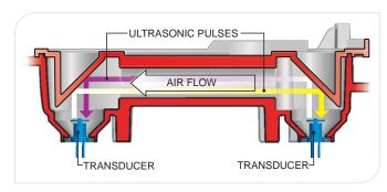
In this application, the ultrasonic flow sensing technology was adapted to monitor air rather than fluids. Two transducers (Blue) are used to continually send signals to each other. One signal travels with the flow (Violet), the other against (Yellow). The time difference between the two signals is used to calculate the rate of airflow within the pipe.
