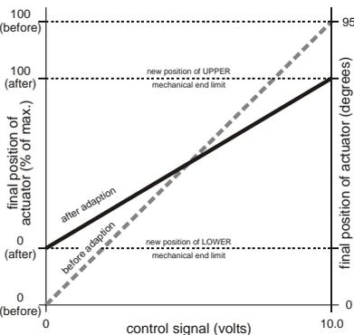
Fig. 6. Adaption (selection switch set to "0...10 V")
