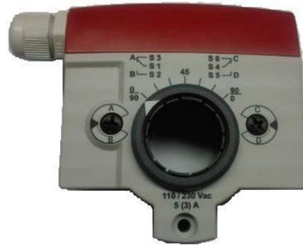
The auxiliary switches are field-installable parts providing two SPDT freely-adjustable switches. (Contact range 5A for resistive, 3A inductive, 110/230Vac)
