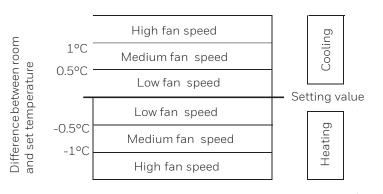
Figure 1. Automatic Fan Speed Control Algorithm
