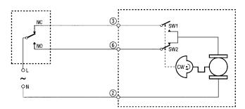
Fig. 3. Logic sequence diagram with 3-wire actuator for SPDT contoller
