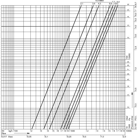
Fig. 9. Valve pressure loss characteristic
