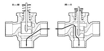
Fig. 2. Fluid flow through 3-way VC valve
