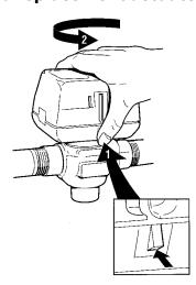
Fig. 8. Latch mechanism
