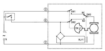
Fig. 4. Logic sequence diagram with 2-wire + common actuator for SPST contoller
