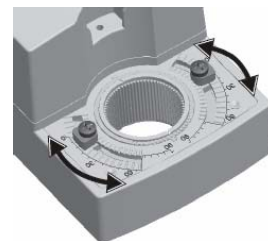
Fig.9. Mechanical end limits
