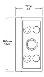
NOTE: The outside enclosure slows the sensor response time to approximately 30 minutes for a 90% step change of CO<sub>2</sub> concentrations.
